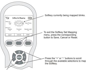
Press the "<" or ">" buttons to move to the previous/next Softkey set. Note that the selection will blink while being mapped.
